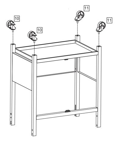
4. Attach the 4pcs wheels (10&11) to the end of frame legs. Note: the 2pcs wheels with brake (10) must be on the same side.
