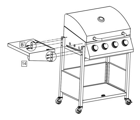
6. LH side shelf (14) is attached to the body with 6 pcs M5 screws (B).
