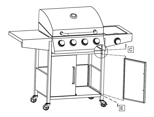
12. Doors are attached to frames' front legs with top and bottom pins (C&E).
