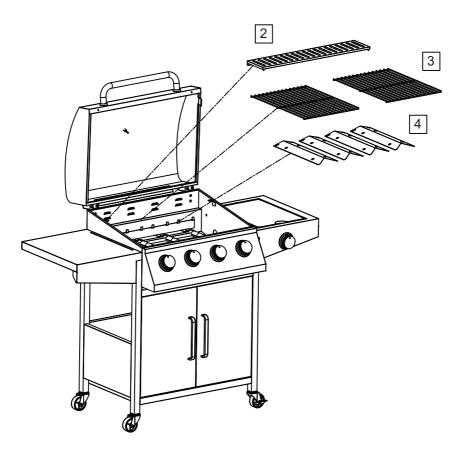
13. Warming grid (2), cooking grids (3) and heat tents (4) are placed into the body.
