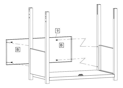
2. Attach the rear panel (9) to the frames with 4 pcs M5 screws (B).
