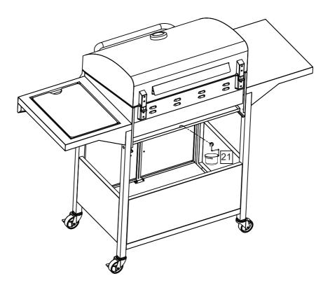
14. Oil cup (21) is attached to the oil pan.
