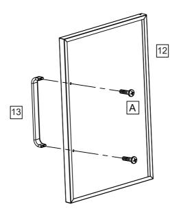
11. Handles (13) are attached to front doors (12) with 4pcs M4 screws (A). Totally 2 pcs doors.
