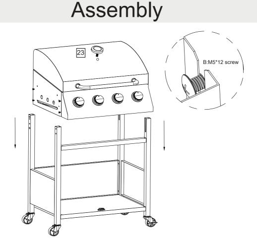
5. Attach 8 \* M5 screws (see diagram). Slide the body (1) onto the frame legs, ensuring the screws are held in the slots on the legs (see diagram). Tighten the screws. Fix Thermometer to lid.
