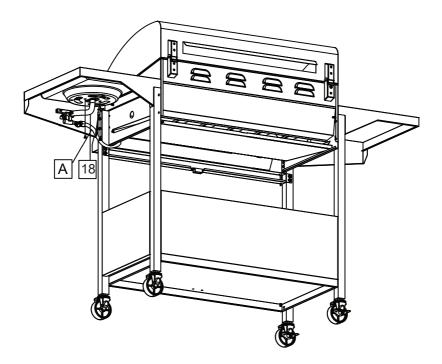
9-1. Side burner (18) is attached into the side burner shelf with 2 pcs M4 screws (A). Insert the tube to valve connector.No need this step for A serial.
