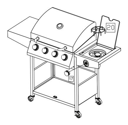
Control knob (17) is attached to side burner's front plate. Grate (20) is placed on the side burner shelf, with the 3 longer legs positioned into the holes to hold it firmly in place. (Not A series grills).
