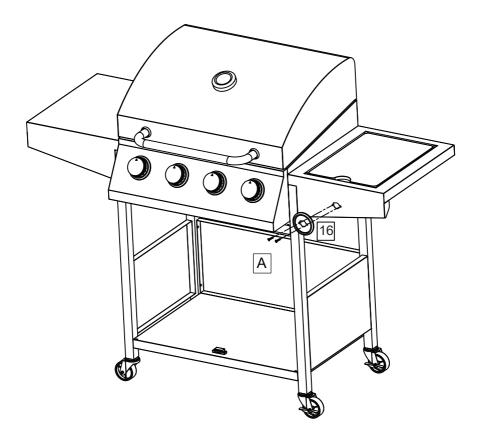
Side burner rotary switch base (16),side burner front plate and side burner valve (inside shelf front plate) are attached together with 2pcs M4 countersunk screws (A). No need for this step for A serial.
