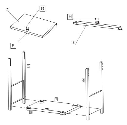
1. Attach the LH and RH frame (5&6) to bottom shelf (7) with 4pcs M5 screws (B).
