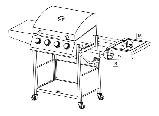
RH side burner shelf (15) is attached to the body with 6 pcs M5 screws (B).
