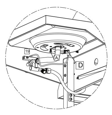
9-2. One end of ignition (19) is attached to the side bunrer shelf with 1 pc M4 screw (A) and 1pc M4 nut (D). The other end is attcheded to the valve connector. No need this step for A serial.
