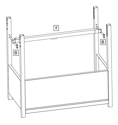
3. Attach the front beam (8) to the front of frames with 4pcs M5 screws (B).
