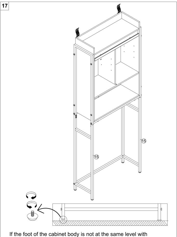
If the foot of the cabinet body is not at the same level with the ground, please rotate the adjusting foot pad of the sole of the foot with your hand to make the feet of the cabinet body level with the ground
